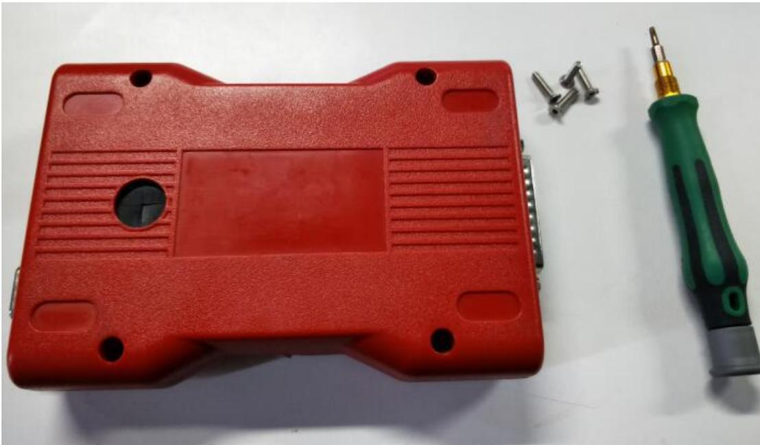
**2.Open the enclosure of the device** : Open the device shell gently by hand, as shown picture below: (Note: Do not force to open it to prevent the wire of the induction coil from being torn off!)
