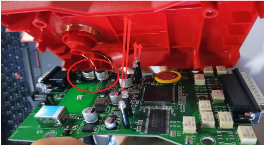
7. **Test function** : Please do not tighten the screws after closing the cover. At this time need to plug USB and 12V to read a key with all direction. If software shows that read successfully, then you could start to tighten screws. As shown in the figure below: (Do not tighten the screws before the reading is successful)
