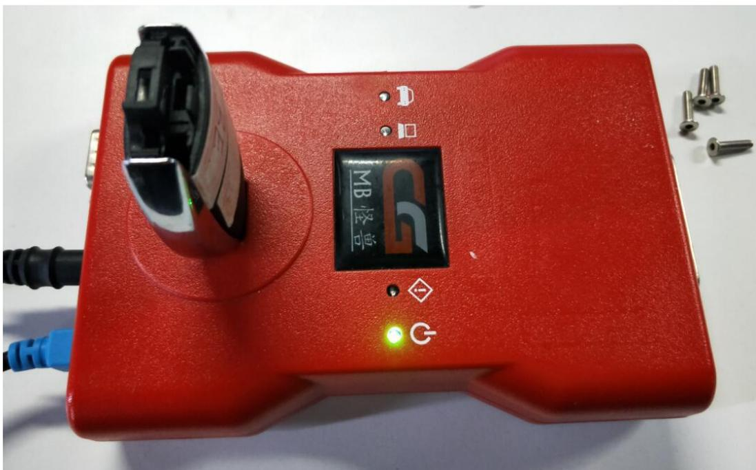
**8. Install the bottom case :** Put the four previously removed screws into the back shell and tighten with a screwdriver. The replacement operation is all completed! As shown below:
