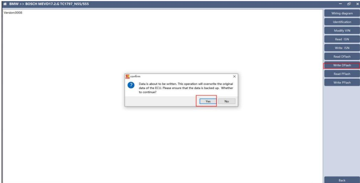
Click "write DFlash" to write the ECU data. Please make sure the data is backed up before writing. The restored data will overwrite the current ECU data. The data can be the data of the current ECU or other ECU of the same type.
