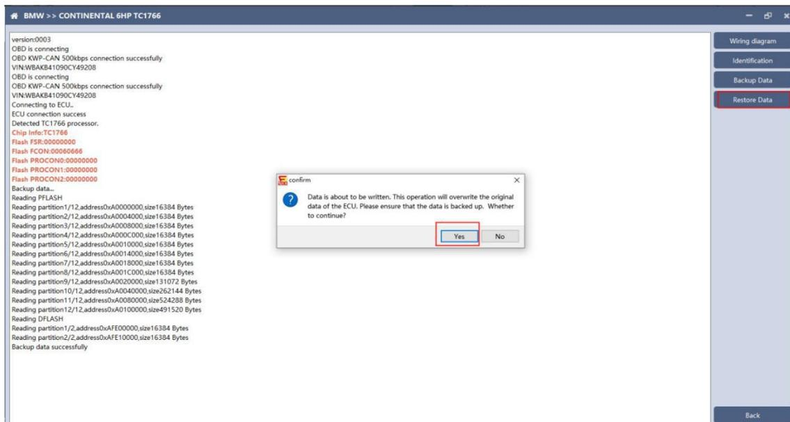
Click "Restore Data" to write the ECU data. Please make sure the data is backed up before writing. The restored data will overwrite the current ECU data. The data can be the data of the current ECU or other ECUs of the same type.
