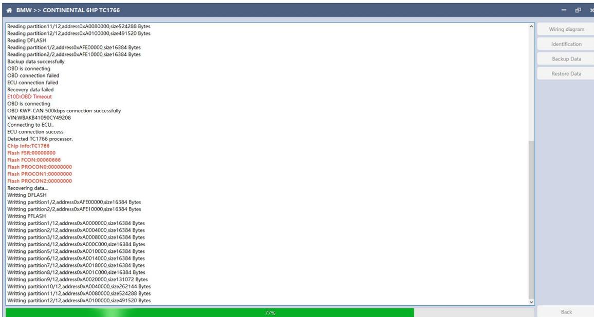
Note: During the data restore process, it is strictly forbidden to disconnect the device from the power or disconnect the device; if the software is unexpectedly shut down or the computer is shut down or
