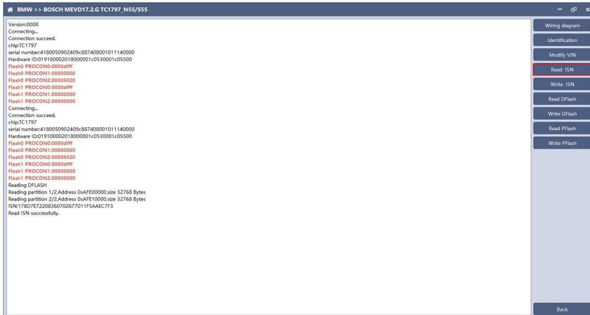
Click the "Read ISN" button to start reading the ISN. Wait for a while to complete the reading of the ISN.
