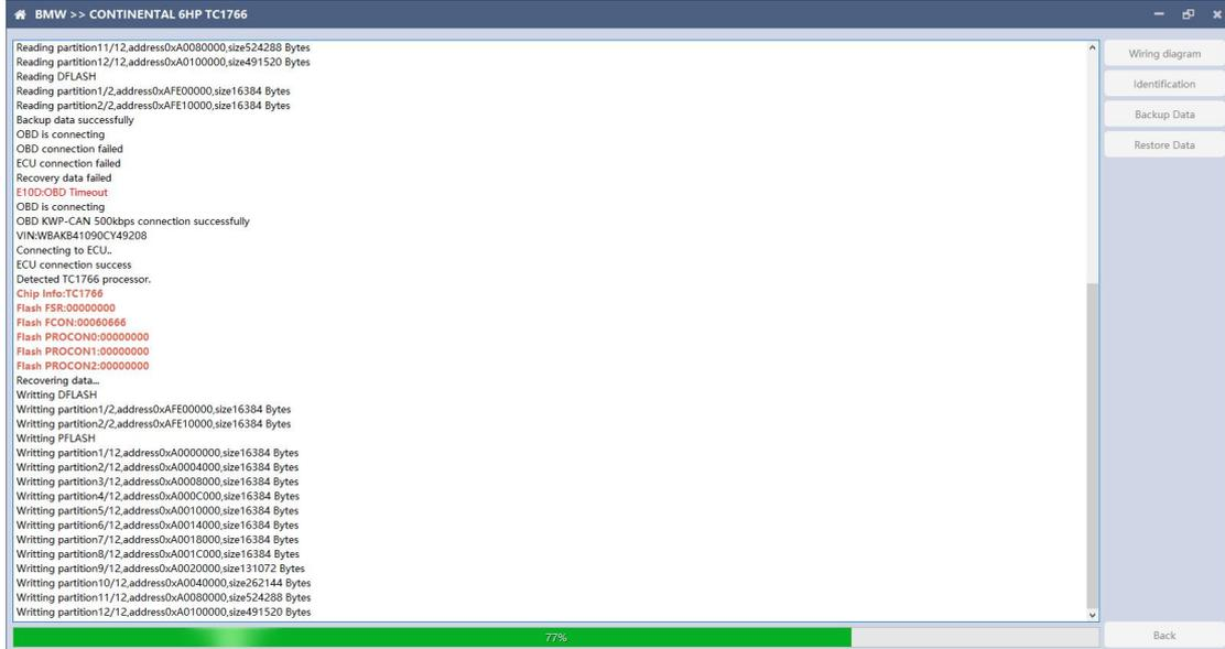
Note: During the data restore process, it is strictly forbidden to disconnect the device from the power or disconnect the device; if the software is unexpectedly shut down or the computer is shut down or crashed unexpectedly during the data recovery process, please do not disconnect the device power or the device connection for 15 minutes , The device can complete the data restore independently.
