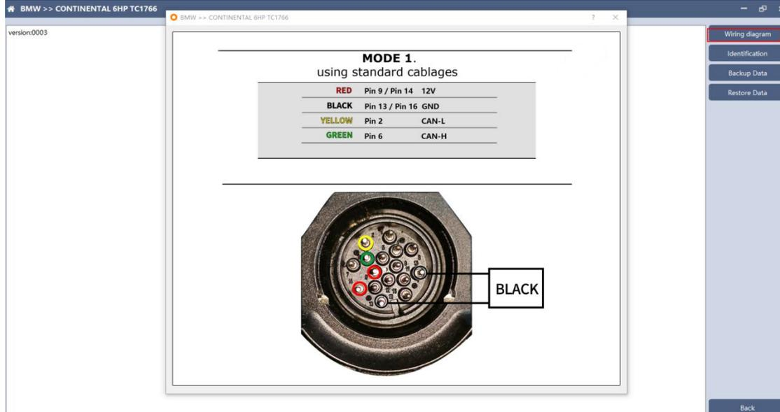
Click the "Wiring Diagram" button to view the ECU wiring diagram, connect the wiring harness correctly according to the wiring diagram, and connect with the device, plug in the device DC12V interface with 12V power supply.
