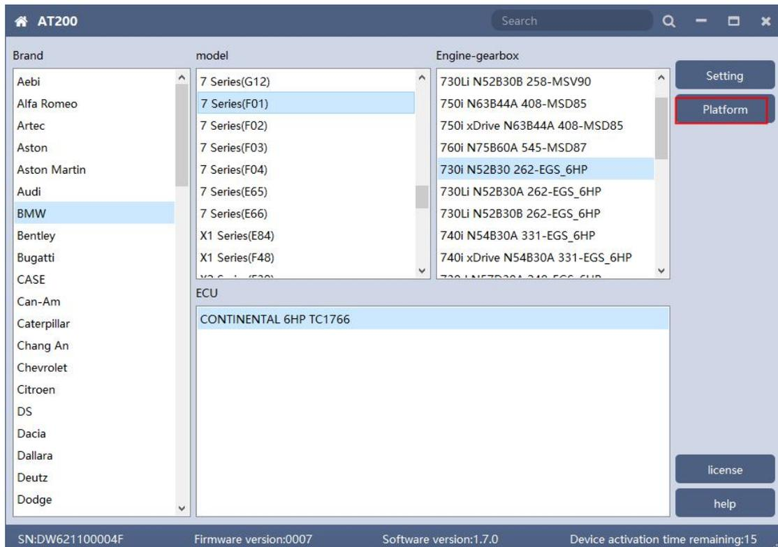
After selecting the correct ECU model, the "Platform" button will appear on the right. As shown in the figure above, click the "Platform" button to enter the ECU operation interface.
