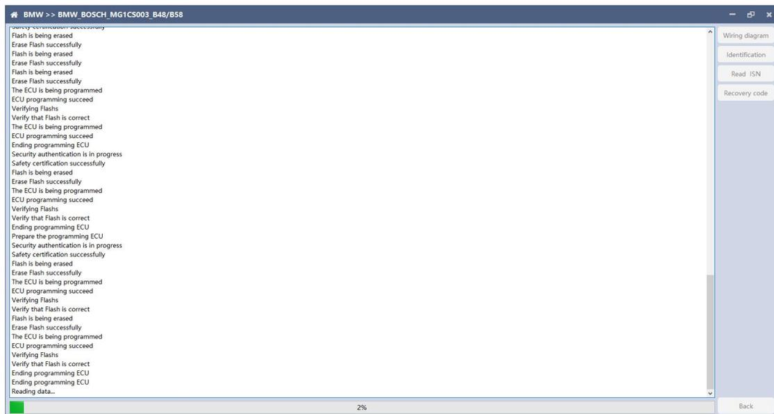
After the programming is completed, if there is a coding file before the ECU programming, the coding recovery will be performed automatically. After programming, the software starts to read data, as shown in the figure above.
